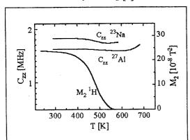
Fig. 1. Temperature dependence M<sub>2</sub> ([110] direction) and C<sub>zz</sub> for the <sup>23</sup>Na, <sup>27</sup>Al in the natrolite powder.
