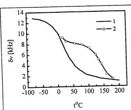
Fig. 1. Linewidth ( $\delta \nu$ ) of the proton resonance vs. temperature in natrolite when the magnetic field  $\mathbf{B}_0$  is parallel to b direction. 1- is the first cases; 2- is the second case (15 hours after heating).
